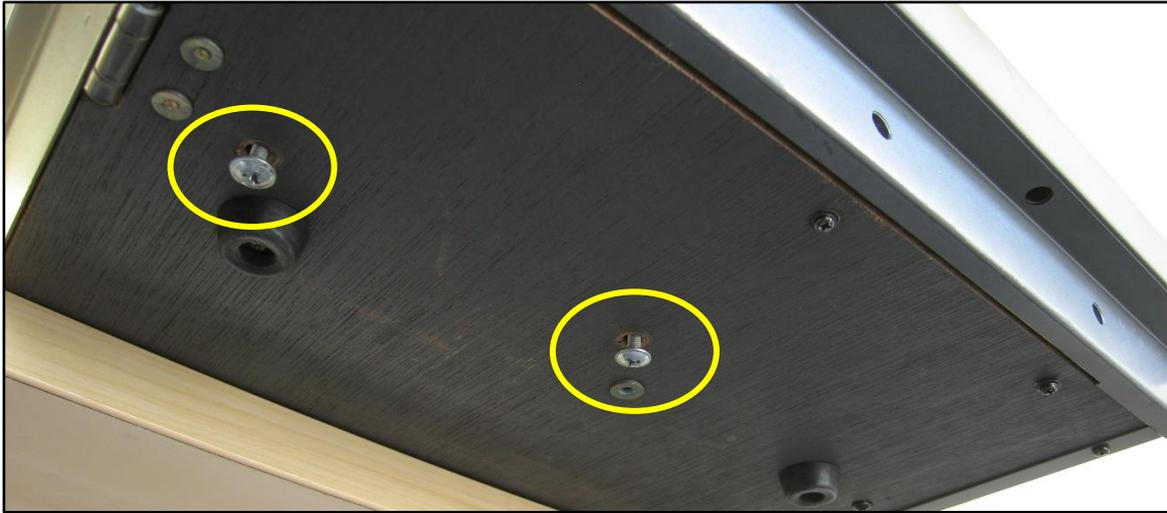
Remove the three screws indicated from both the left and right hand side end cheeks.
