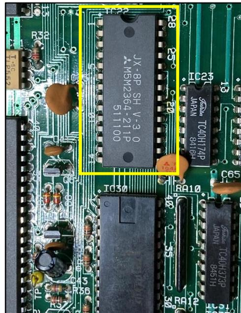
On v2 main boards it is likely to be socketed however on v3 main boards it is likely to be soldered directly to the board. If this is the case, carefully de-solder the 28 pins and remove the IC.
